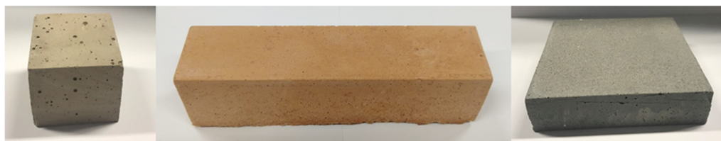
Figure 2. Examples of geopolymer test specimens: cube for determination of compressive strength ( left ), prism for determination of flexural strength ( middle ), and plate for determination of thermal conductivity and bulk density ( right ).
