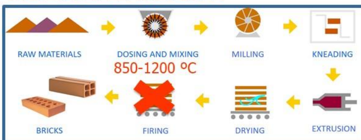
Current brick manufacturing process
